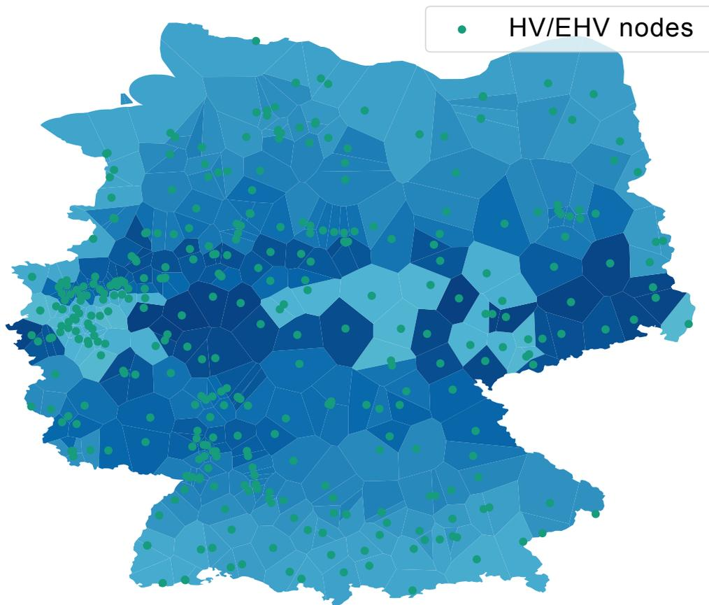
**Figure 3.15:** Voronoi polygons and the corresponding HV/EHV nodes
