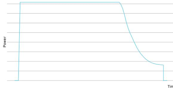
**Figure 3.12:** Schematic charging profile of an EV
