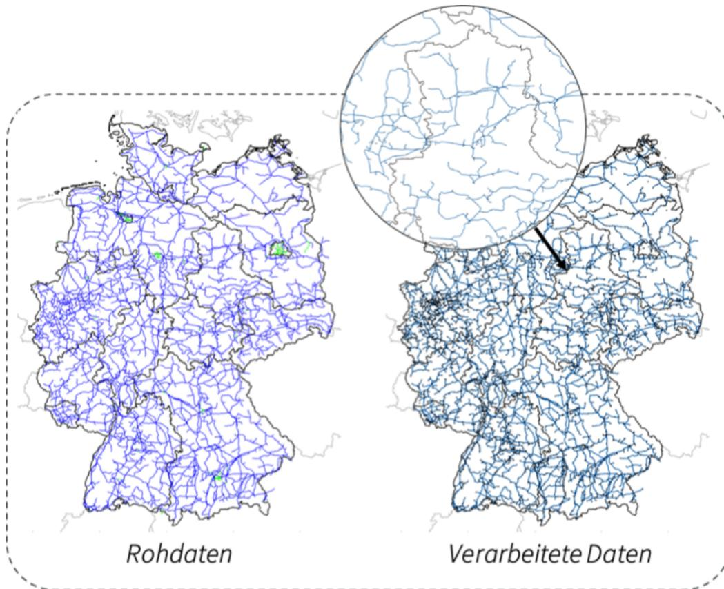
**Figure 3.6:** Georeferenced data for the HV grid
