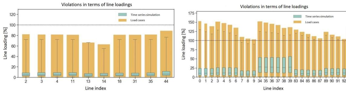
**Figure 5.5:** Comparison of the maximum line loadings based on all defined calculation cases (except n-1) and the annual time series simulations exemplary for the urban LV grid (seen left) and suburban MV grid (seen right) in case of scenario 1
