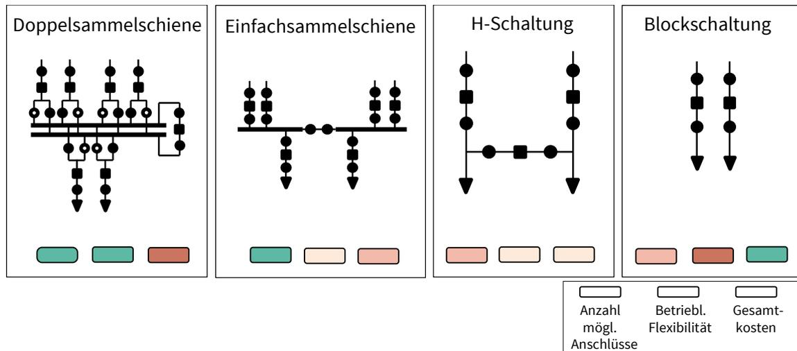
**Figure 3.9:** Station concepts in the HV level
