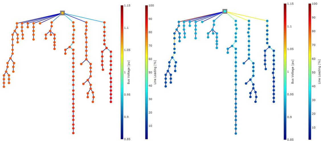
**Figure 4.22:** Picture of the LV grid LV3 with calculated bus voltages and line loadings displayed as heat map for scenario 1 (see left) and 2 (see right)
